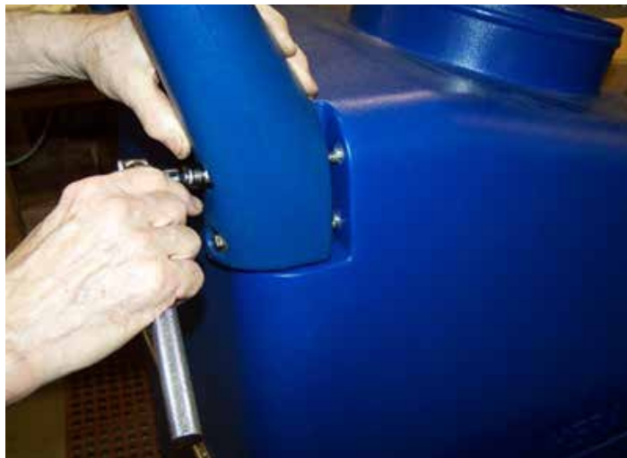
It must be installed with the 4 bolts provided and your 1/2" socket wrench or nut driver.
