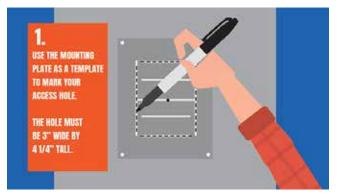
When the proper location for the UVC Max 25 has been selected, use the duct board mounting plate (5" x 7" overall) to draw lines where the duct board must be cut, 3" wide by 4-1/4" tall hole. (Figure 1)
