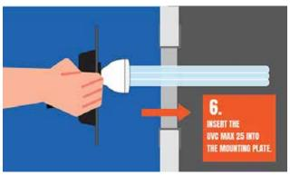
The mounting plate is now ready for the UVC Max 25 to be installed in the same manner it would be installed into a metal duct. (Figure 6)
