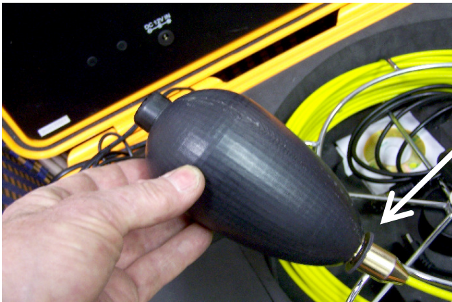
VIS Camera Head Installed in the Float with the Retaining Washer installed on the cable
