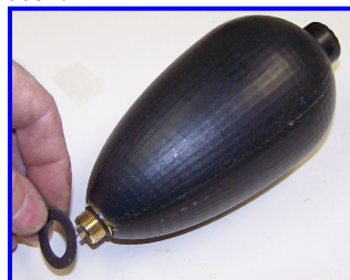
Install Washer over Threads on Rear of Camera
