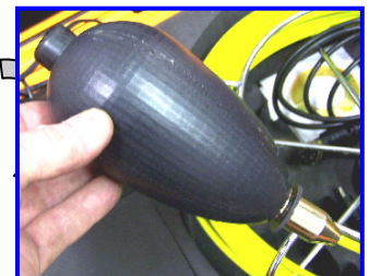
Screw Camera with Float back on to the Insertion Cable Connector
