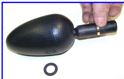
Insert Back end of Camera into Larger end of Float
