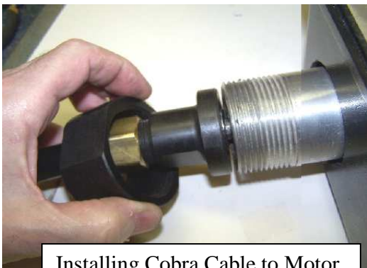
Installing Cobra Cable to Motor Box coupler.
